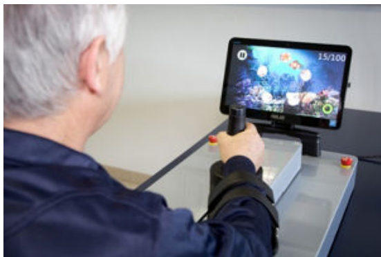
Figure 12 - ICon, an adaptive system for the intensive rehabilitation of neurological patients with upper limb disabilities
